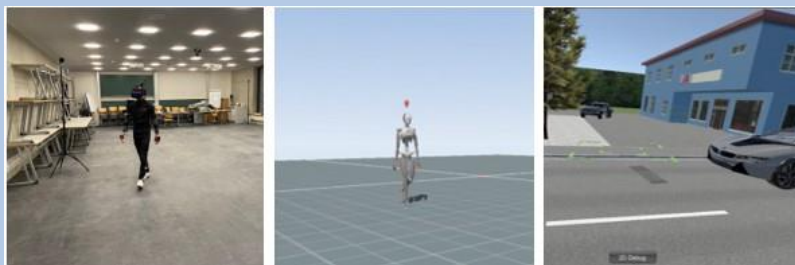
Figure 1: Overview of the setup of the motion-capture studies in subproject 1: test person in the XSens motion-capture suit (left), result of the motion-capture in the software (center), view of the test person in VR (right). Source: THI
