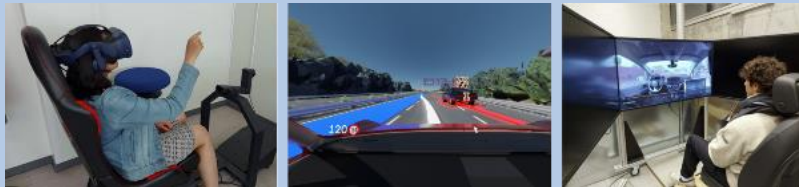
Abbildung 3: . Examples from the user studies in sub-project 2: Driving simulation and virtual reality studies can be used to investigate new display concepts for automated driving, for example regarding acceptance, trust and the general user experience. Source: THI
